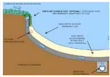
Principal drawing of Capillary Concrete system with optional Capillary Bunker Edge.
